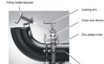
Aligning screws Clamping feet lock screw
